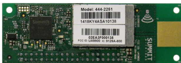
Summit SD TX Module Top View
